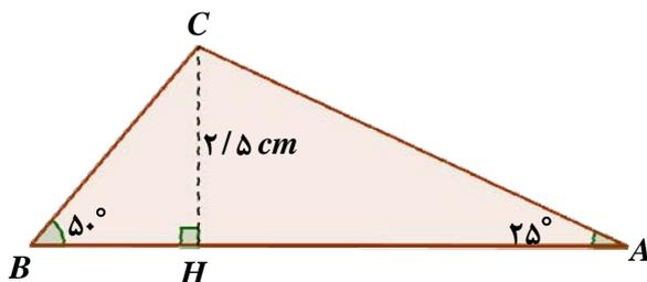
$$\begin{cases} \Delta AHC : \tan 25^\circ = \frac{CH}{AH} \Rightarrow 0/47 = \frac{2/5}{AH} \Rightarrow AH = 5/32 \text{ m} \\ \Delta BHC : \tan 50^\circ = \frac{CH}{BH} \Rightarrow 1/19 = \frac{2/5}{BH} \Rightarrow BH = 2/10 \text{ m} \end{cases}$$
